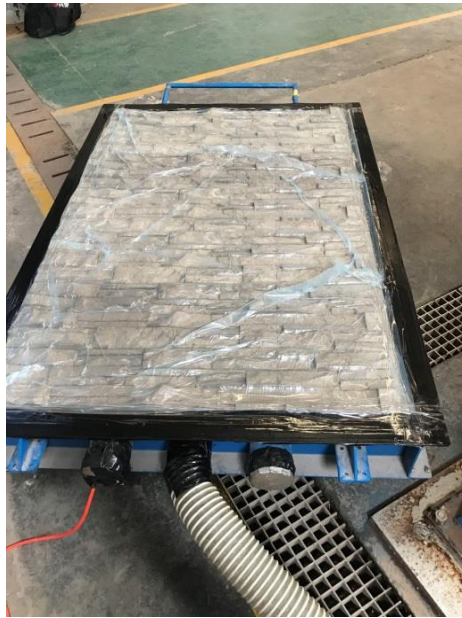
Fig.5 Positive load test set-up
