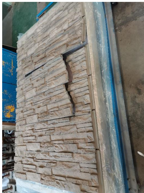
Fig.4 The typical mode of failure on negative load test
