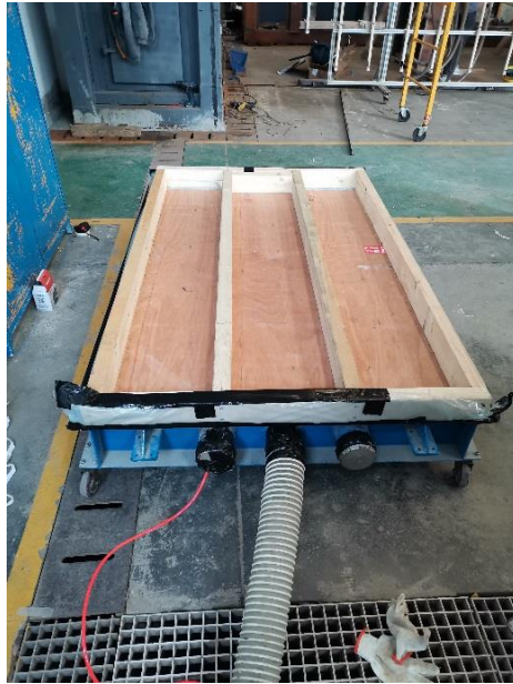
Fig.3 Negative load test set-up
